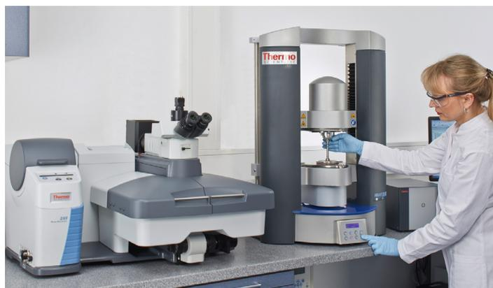
**Figure 1:** Combination of a Thermo Scientific HAAKE MARS with a Thermo Scientific DXR Raman Microscope.
