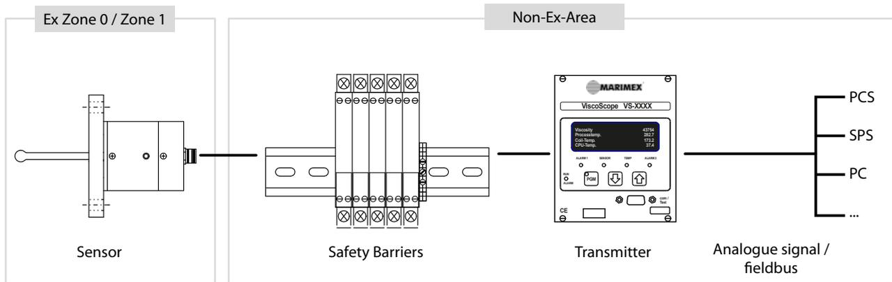
Typical system design for installation in Ex-Area
