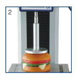
In a compression test, the load cell acts just like an upside down laboratory balance. Data collection can be "triggered" to begin when the sample's surface is detected giving a constant start point to repetitive tests.
