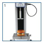
The texture analyzer's crosshead moves in either an up or down direction to compress or stretch a food sample. The moving crosshead is fitted with a load cell to measure the foods force response to the deformation.
