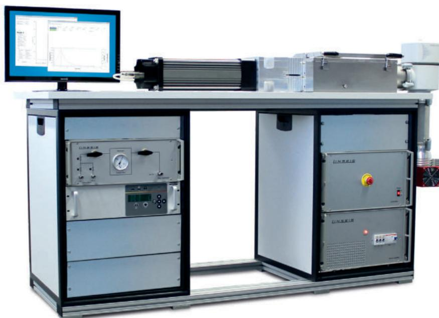
Quenching/Deformation Dilatometer L78 RITA/Q/D/T
