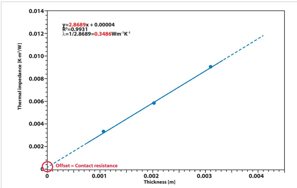
Measurement of the thermal impedance (thermal conductivity) of a 25mm x 25mm Vespel™ sample at 50°C ( $T_H=70^\circ\text{C}$ ,  $T_C=30^\circ\text{C}$ ) and a contact pressure of 1 MPa. Three different samples with a thickness between 1,1 mm and 3,08 mm have been measured in order to determine the apparent thermal conductivity and thermal contact resistance (using linear regression).
