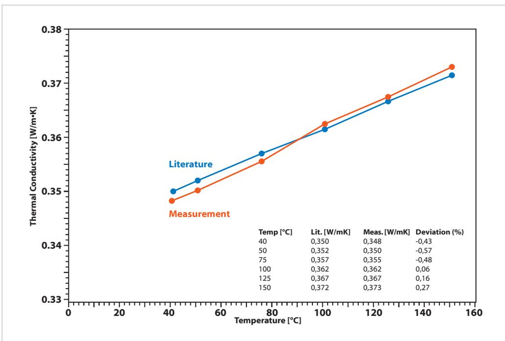
Plot of the temperature dependent apparent thermal conductivity of a 25mm x 25mm Vespel™ sample between 40°C and 150°C and a constant contact pressure of 1 MPa.
