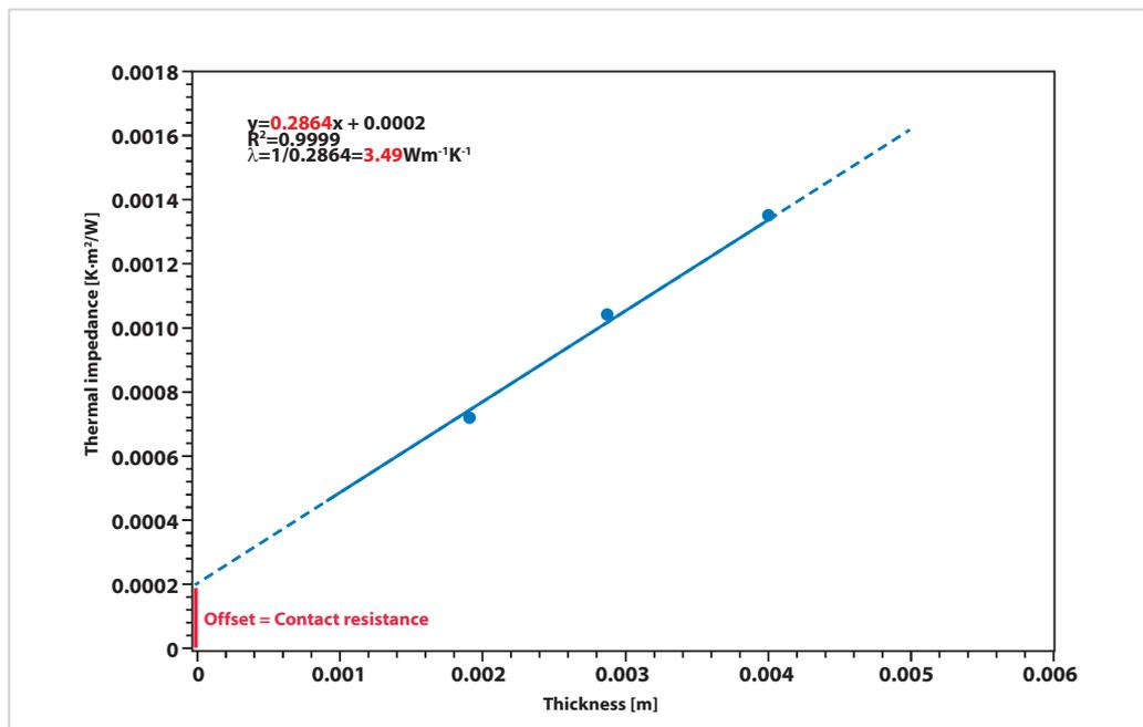
Measurement of the thermal impedance (thermal conductivity) of a 25mm x 25mm thermal conductive pad (sample type 2) at 50°C ( $T_H=70^\circ\text{C}$ ,  $T_C=30^\circ\text{C}$ ). Three different samples with a thickness between 2.01 mm and 3.02 mm have been measured in order to determine the thermal contact resistance (using linear regression).
