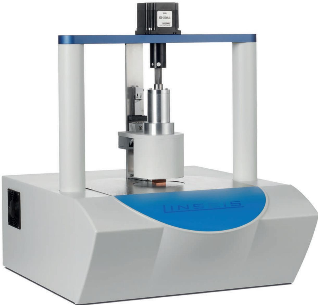
**Automatic pressure adjustment using electric actor (up to 8 MPa)**
