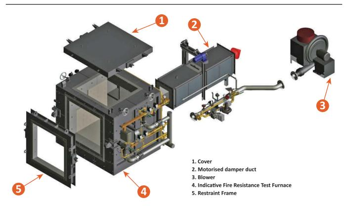
1m × 1m Furnace, 2 burners, based on an upright furnace position are installed on the opposite side of the furnace wall. A third burner is installed near the top of the furnace. Each burner is designed to use liquefied petroleum gas and all necessary flame safety systems, intermittent pilot systems, and temperature sensors are incorporated.
