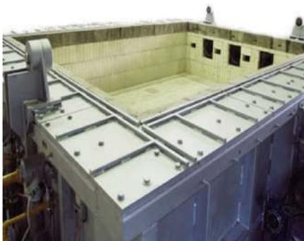
The **FTT** Horizontal Fire Resistance Test Furnace
