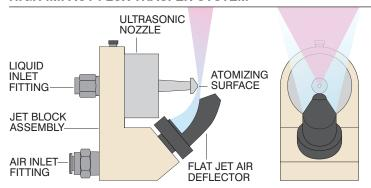
FLUX APPLICATION - Flux is supplied from a closed pressure reservoir to the ultrasonic nozzle. The flux reservoir includes a level sensor to alert the operator to a low level flux condition. The flux is atomized into a fine mist at the tip of the non-clogging, large-orifice ultrasonic nozzle which is reciprocated below the PCB, directing flux upward.
