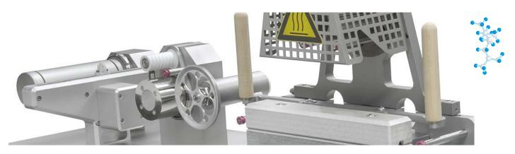
The lateral moving speeds of the traverse guides on both units are (in)dependently controlled to generate a variety of filament overlap pitch patterns. The pitch between adjacent fibres can be controlled within 0.1 mm to 4.0 mm. The units accommodate 0.75 mm cardboard bobbins. The fibre heating options of the conditioning unit consist either of a hot shoe, which heats the fibre by radiation, or optionally, a heated metal cylinder, which heats the fibre by conduction.
