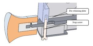
Die retaining plate is detachable by removing stop screw, facilitating cleaning.
