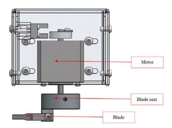
It is mounted under the cylinder. Step motor drives blade to rotate and cut the sample. Blade has high stiffness, easy to cut and clean.
