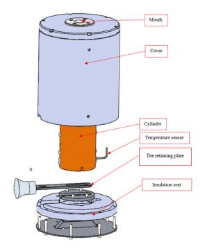
In order to ensure the uniform temperature of the cylinder, the external part is processed with 70mm copper in diameter to ensure the maximum uniformity of the internal temperature.
