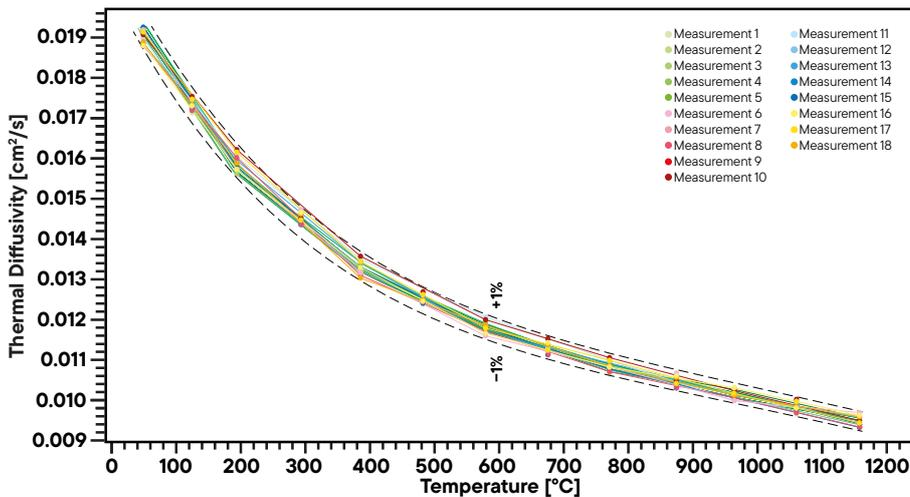
Pyroceram, a glass ceramic trademark of Corning used as a standard material in various applications, has been measured using the LFA L51 1250 to show the reproducibility of thermal diffusivity values. In total 18 measurements were performed with 18 samples that were cut out of one bulk block. Each sample was measured separately and the result shows a spread in the result that is in a range of +/- 1% in a temperature range up to 1160°C.
