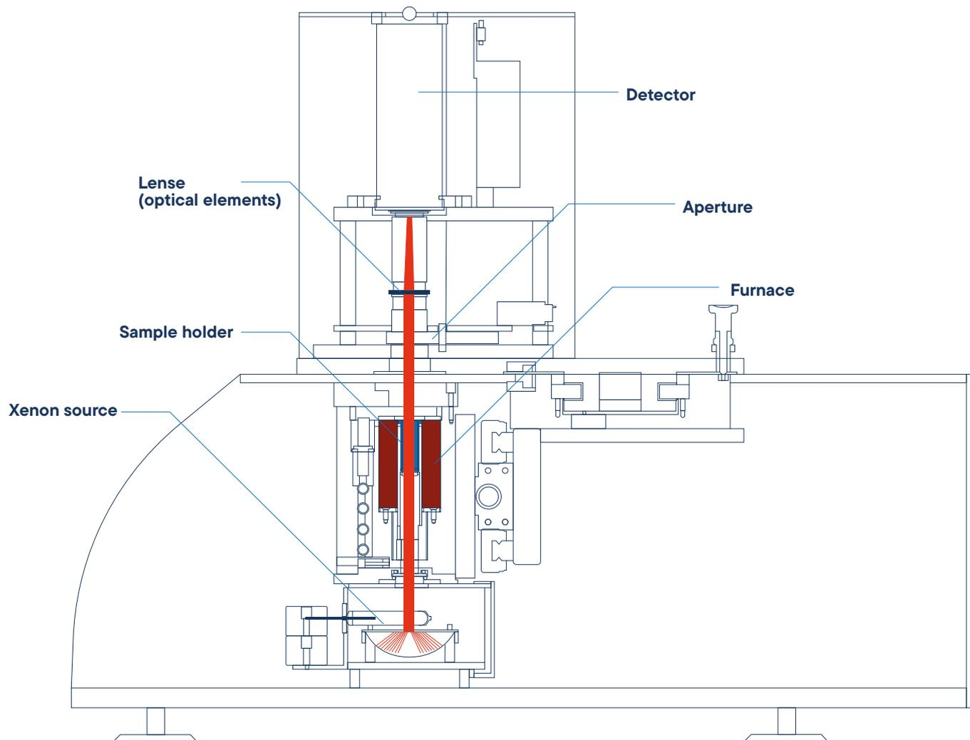
The Linseis **LFA L51 1250** features a vertical configuration with the detector positioned above the sample and the Light Flash source below. This design facilitates straightforward handling and optimal measurement outcomes. The five micro-heaters heat ultra-fast, which minimizes the total measuring time and increases the throughput.
