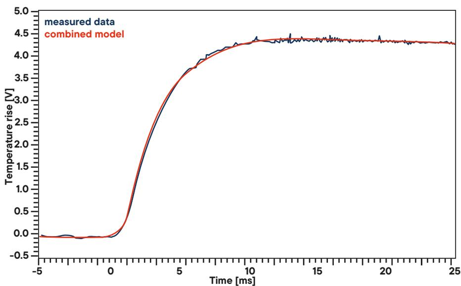
Temperature rise of a graphite sample (length 1.11 mm, half time rise 4.37 ms). The combined model curve is fitted to the data points.
