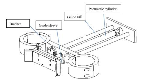
Push out the broken sample from test area, and clean the lower plate simultaneously.
