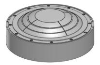
Fully enclosed double spherical structure improves flexibility, makes the stress more uniform, and improves the accuracy of loading force, ensures the concrete sample fractures uniformly.
