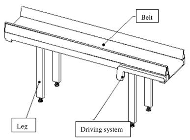
The collecting line is used to carry broken samples.
