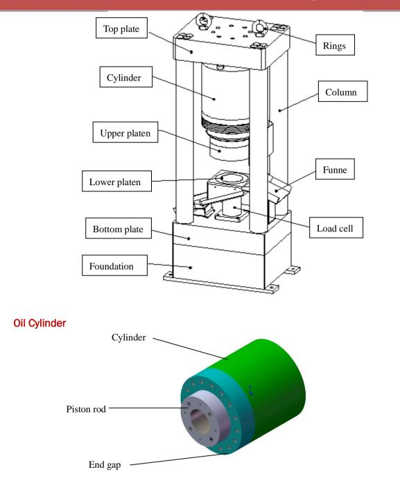
The main oil cylinder loading in both directions; piston rod plating with Ni&Cr, coating thickness of 0.1mm, to enhance anti-corrosion property and abrasive resistance. One body casting piston to ensure impact resistance.
