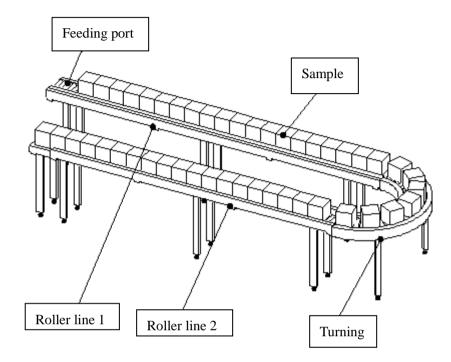
The charging line is used to place the sample and feed it to the port automatically.
