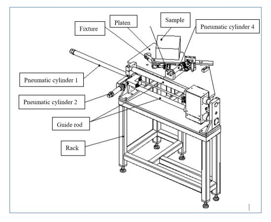
Use several pneumatic cylinders linkwork to push the sample into the testing machine to do the test from the roller line.
