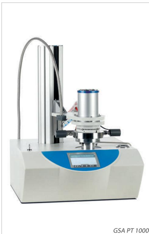
The adsorption or desorption of various gases by materials like catalysts or porous structures is one special, but very frequently asked application on thermo-balances. In general, there are two ways of monitoring adsorption and desorption, the volumetric sorption, where a definite amount of gas is brought into a sample chamber and the pressure change provides the information, and the gravimetric sorption, where the mass change of the sample is analyzed. With
