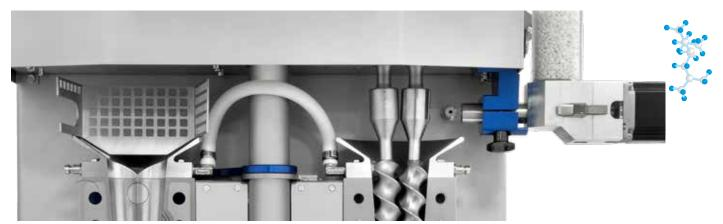
instrument fits in a fume cupboard. Its new, state-of-the-art robust, precise and reliable continuously digitally variable 24 bits motor drive enables accurate monitoring of the screw torque. The result, easy accurate upscaling to any larger parallel twin screw extruder, furthermore, it requires less service by its improved design.
