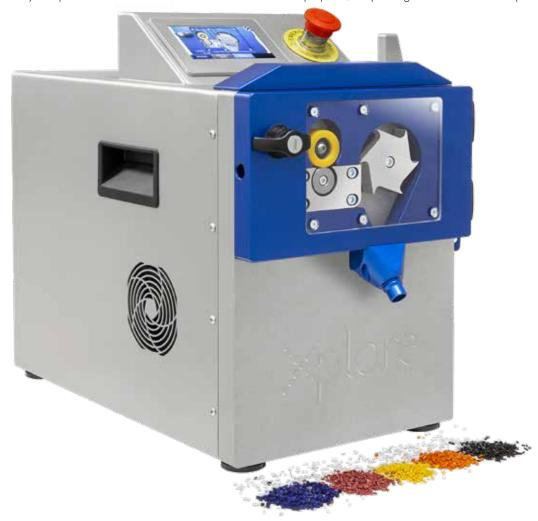
The polycarbonate transparent front window gives you an inside look of the pelletizing process. An optional water bath enables you to cool the polymer strand before the initial cutting (pelletizing) step.
