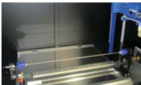
Electrospinning of tube fibers for artificial blood vessels with a special mandrel collector
