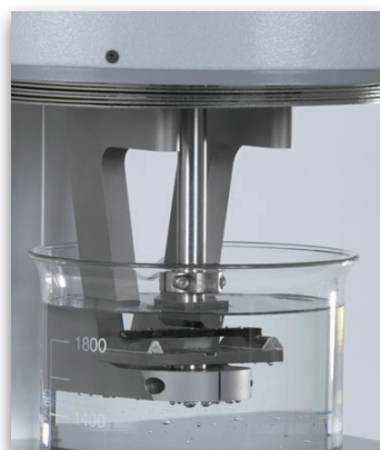
Composite material tested in a solvent bath.
